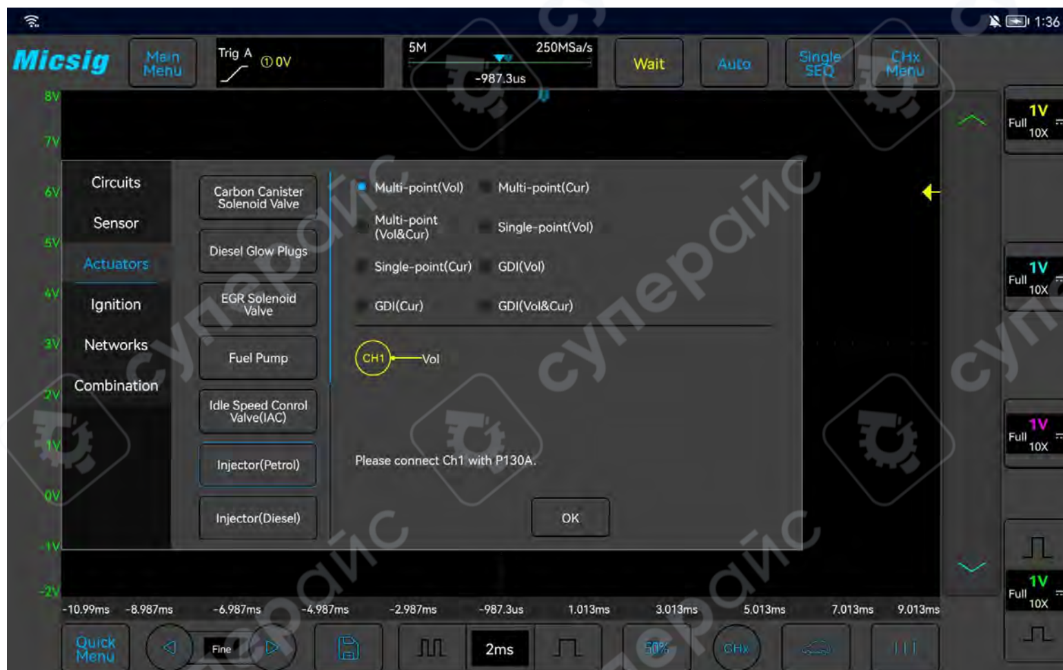
Figure 3-35 Injector (Petrol) Test
