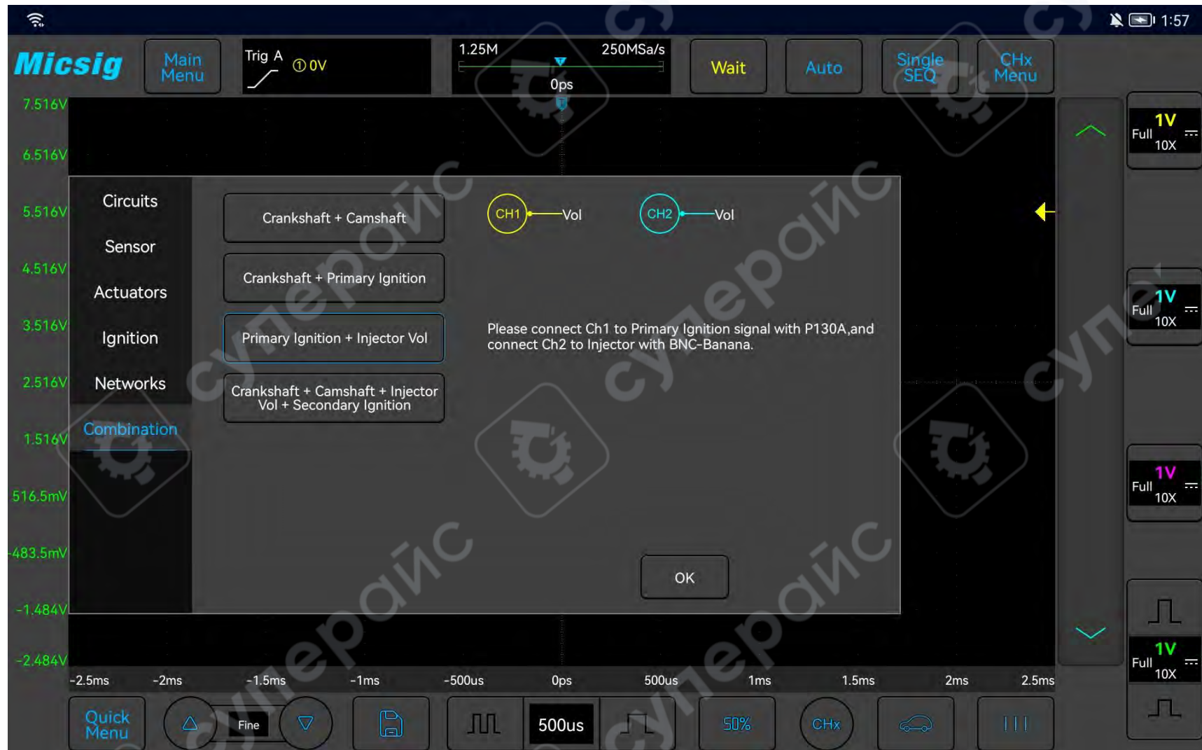
Figure 3-57 Primary ignition + Injector voltage
