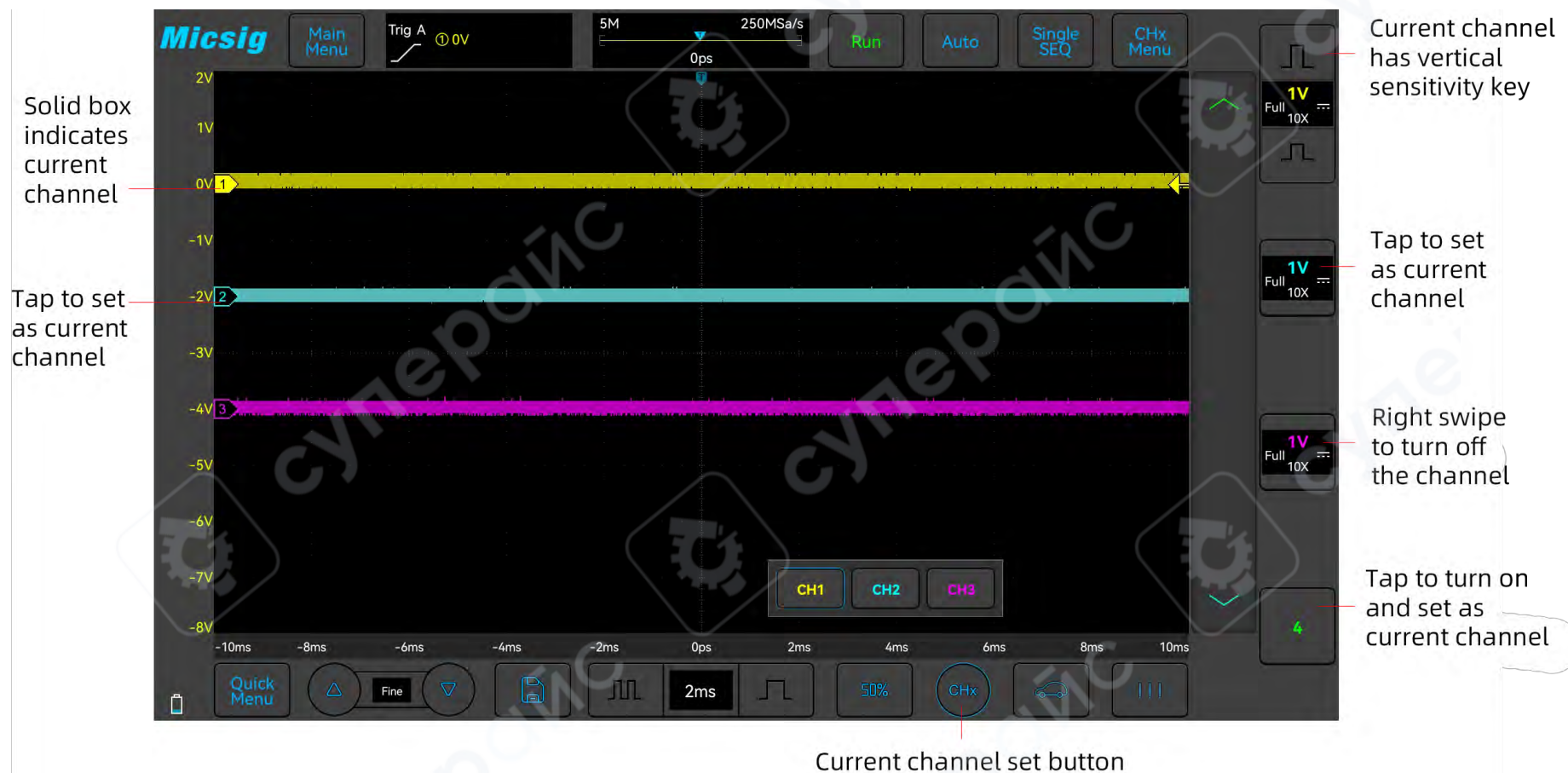
Figure 5-4 Channel Open, Close and Switching
