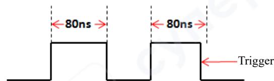
Figure 6-18 Trigger Time T \neq 80\text{ns}
