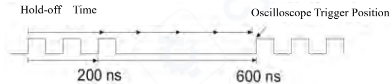
Figure 6-9 Trigger Hold-Off Time
