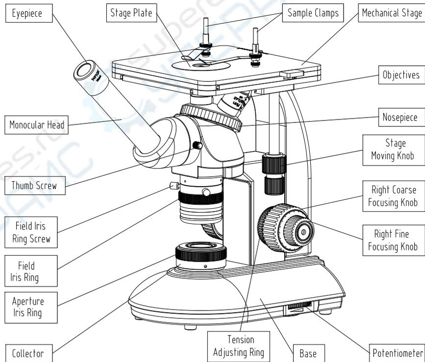
Fig.2 MDJ100 Metallurgical Microscope
