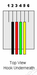
When testing RJ11 phone cables: Tester will test each pin sequentially. Green LED will illuminate for phone cables starting at pin 1 and ending at pin 8. Cable is GOOD when all green LED's light up in sequential test order:
