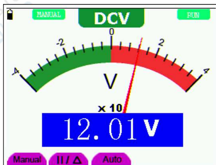
Figure 33: Automatic/Manual Range Adjustment
