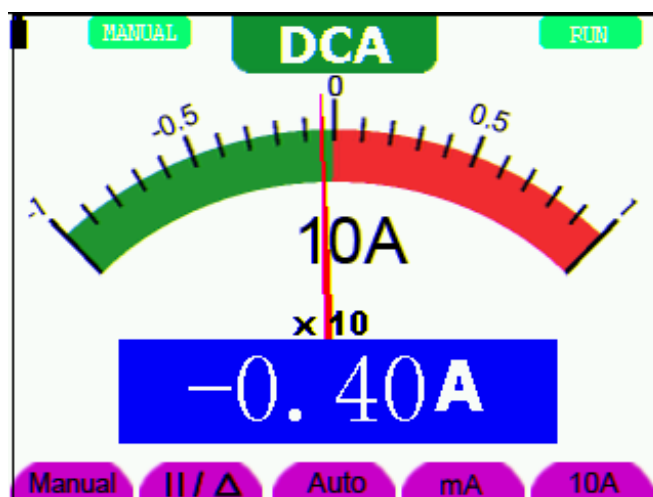
Figure 28: DC Current Measurement for 10A
