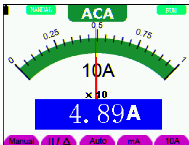
Figure 30: AC Current Measurement for 10A
