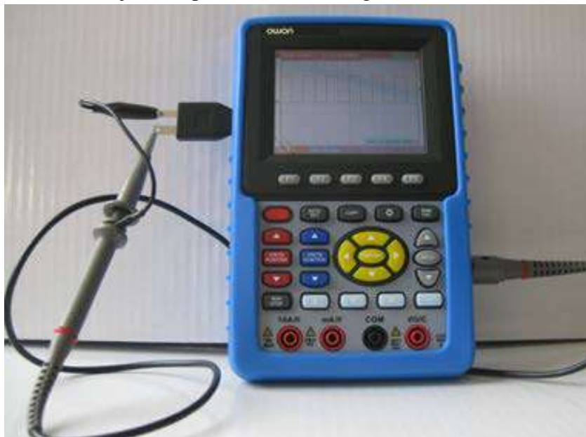
Fig.3. The connection of Square-wave test signal
