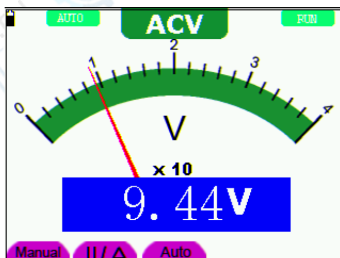
Figure 26: AC Voltage Measurement
