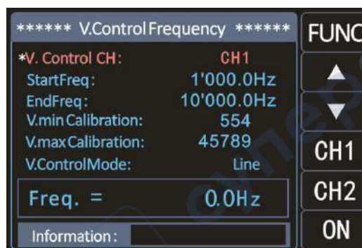
Figure 3-6-1 Voltage Control Interface
