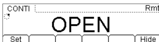
Figure 2-26 Continuity Testing Interface
