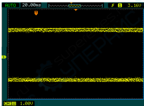
Figure 2-64 Adopt peak detect acquisition, signal contains envelope
