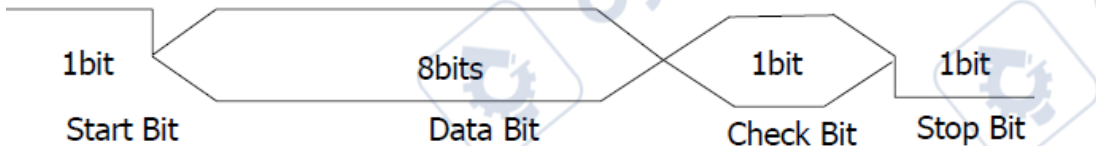
Figure 5-13 Schematic Diagram of RS232 Protocol
