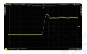
UltraVision: multi-level intensity grading display (256-level)
