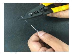
Use the fiber stripper to remove the fiber cladding (about 5 cm).
