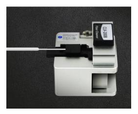
Open the fiber holder and the cover, and carefully move fiber from cleaver to fusion splicer.
