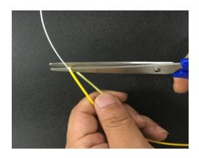
Use the fiber stripper to cut off the kevlar.
