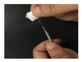
Use the alcohol-impregnated gauze or cleaning wipes to clean the bare fiber.
