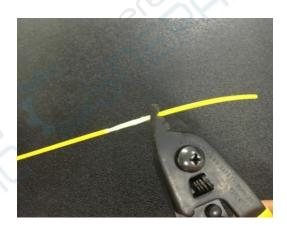
Use the fiber stripper to remove the buff tube (about 25 cm).
