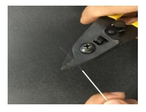
Use the fiber stripper to remove the fiber coating(about 5 cm).
