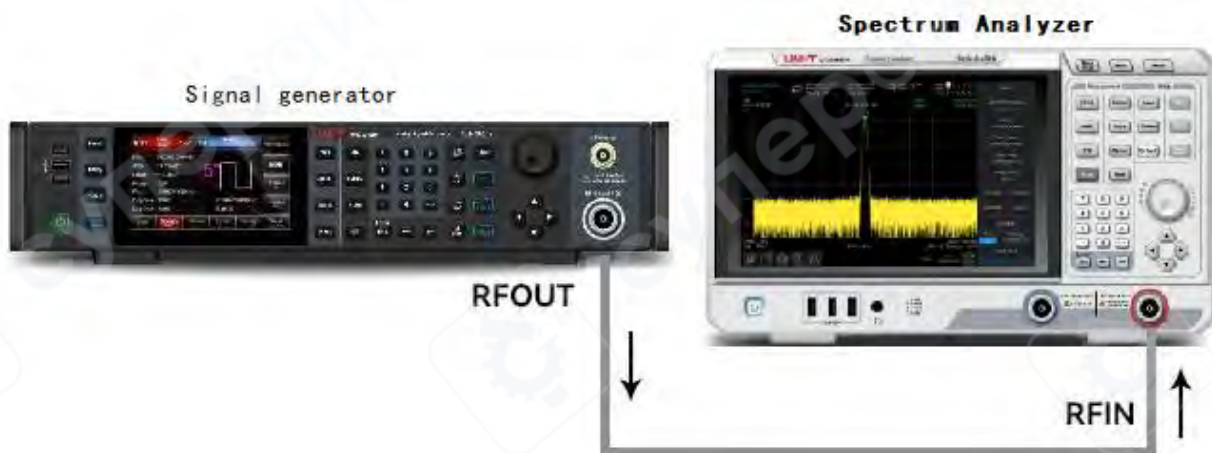
Figure 3-10 Instrument Setting for Acquire Single Signal
