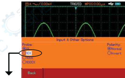
Figure 2-11 Setting the probe ratio
