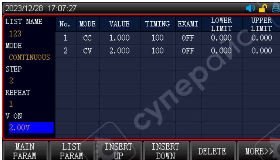
Figure 7-2-13 Automatic List Test Setting Interface
