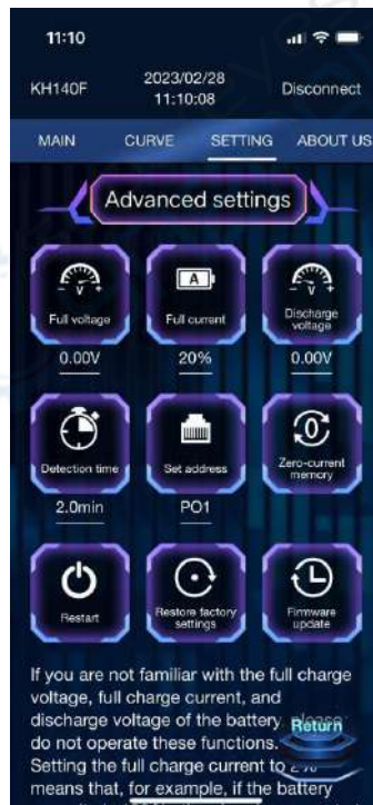
Figure 3-4-73 System Settings - Advanced Settings
