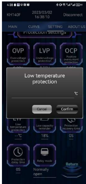
Figure 3-4-43 LTP low temperature protection
