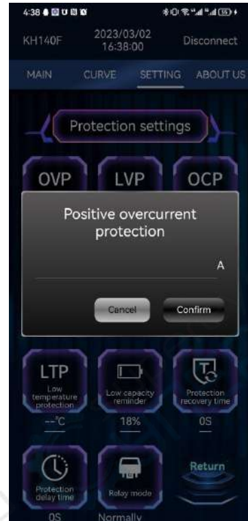
Figure 3-4-39 OCP discharge overcurrent protection
