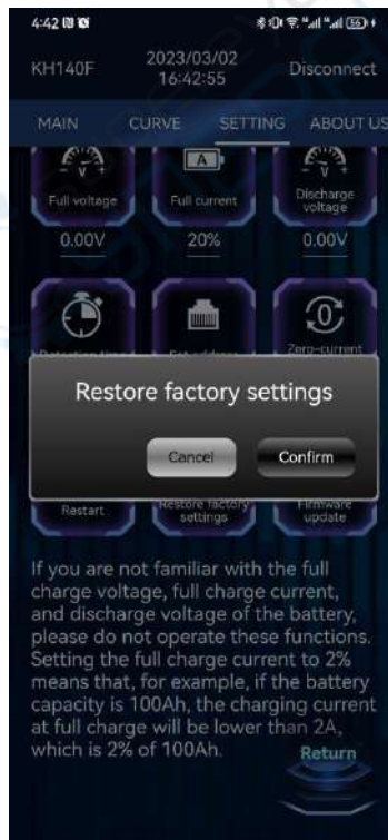
Figure 3-4-55 Restore Factory Settings
