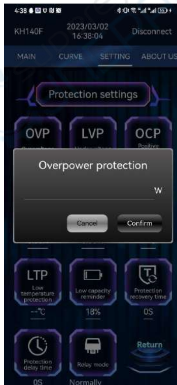
Figure 3-4-41 OPP overpower protection
