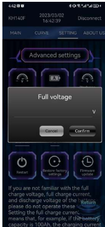
Figure 3-4-48 Full charge voltage
