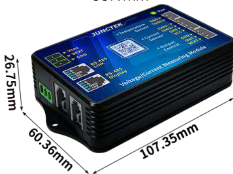
Dimension of measurement module
