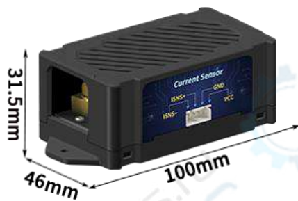
Dimension of the 100A sampler
