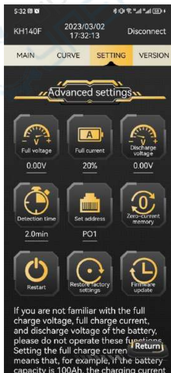
Figure 3-4-65 System Settings - Extended Functions
