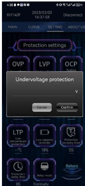
Figure 3-4-38 LVP undervoltage protection
