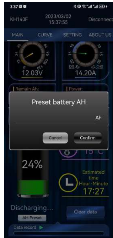
Figure 3-4-21 Preset battery capacity
