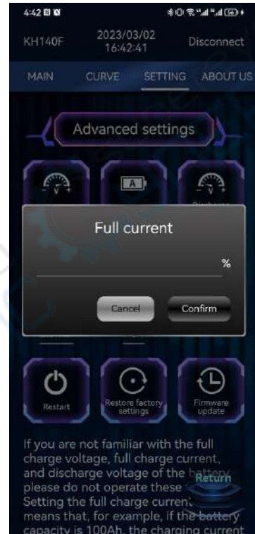
Figure 3-4-50 Full charge current
