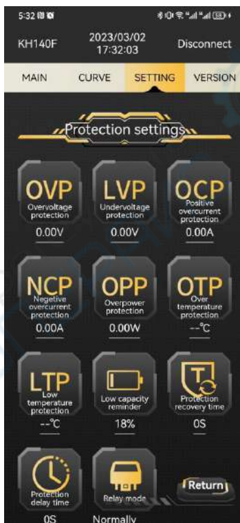
Figure 3-4-64 System Settings - Protection Function
