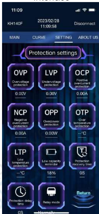
Figure 3-4-72 System Settings - Protection Function
