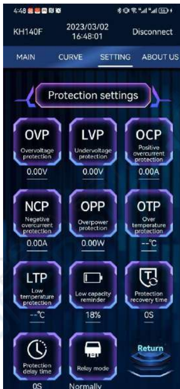
Figure 3-4-7 System Settings - Protection Settings
