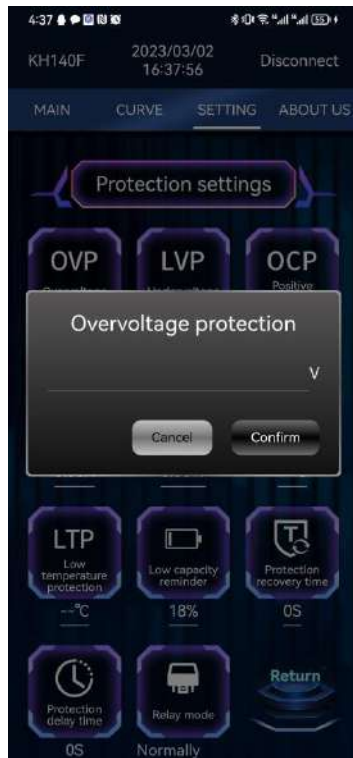
Figure 3-4-37 OVP overvoltage protection
