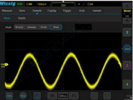
Figure 11-5 Sine Wave with Burr
