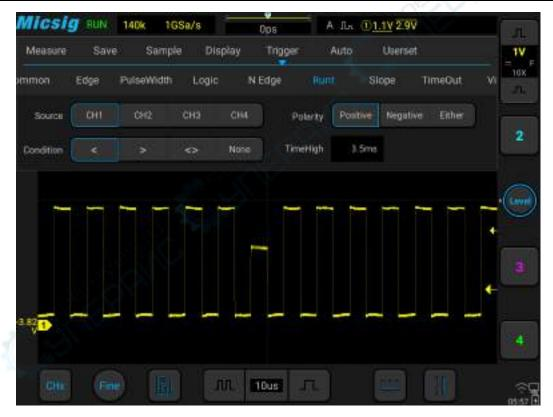
Figure 6-25 Runt Trigger Setting Menu
