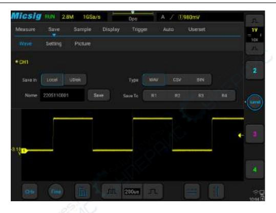
Figure 8-5 Save CH1 Reference Waveform Interface
