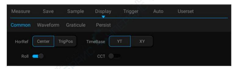
Figure 4-7 Roll Mode On/Off
