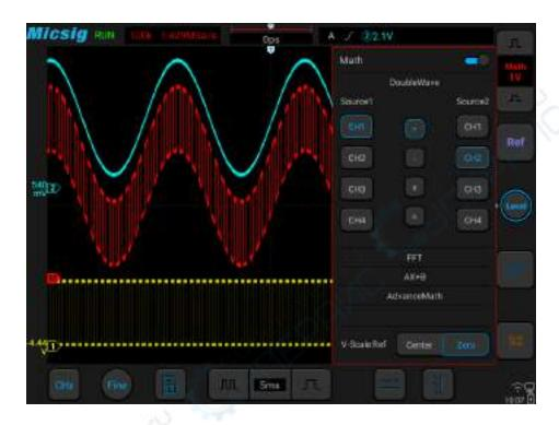
Figure 9-2 Mathematical Operation of CH1 adding CH2
