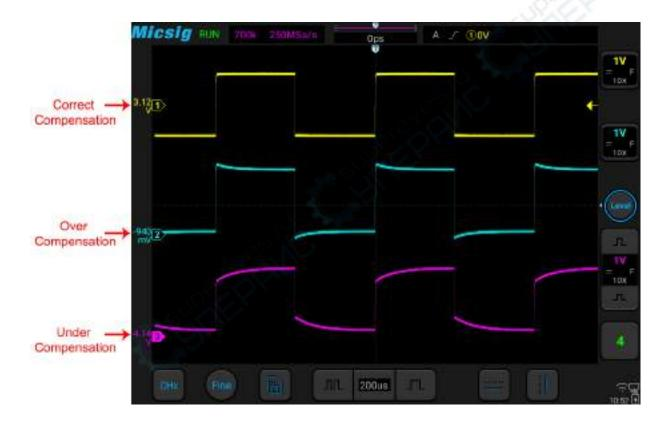
Figure 2-14 Probe Compensation
