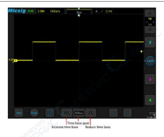
Figure 4-3 Adjust the Horizontal Time Base
