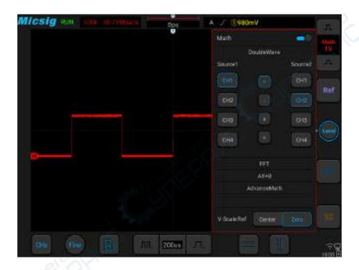
Figure 9-1 MATH Channel Waveform
