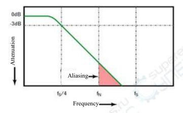
Figure 11-3 Sampling Rate and Oscilloscope Bandwidth
