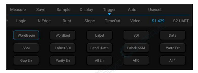
Figure 12-27 ARINC429 Trigger Mode Configuration Menu
