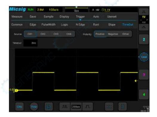
Figure 6-29 Time-out Trigger
