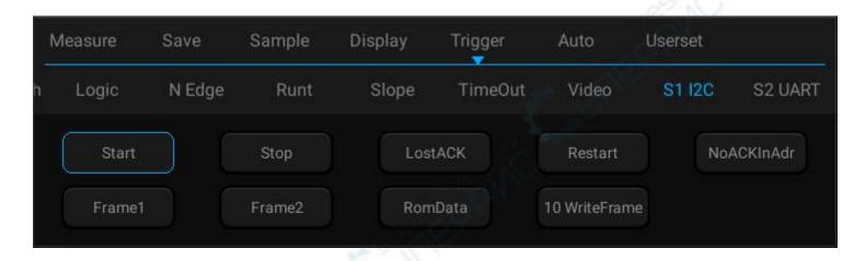
Figure 12-23 I2C Trigger Mode Configuration Menu
