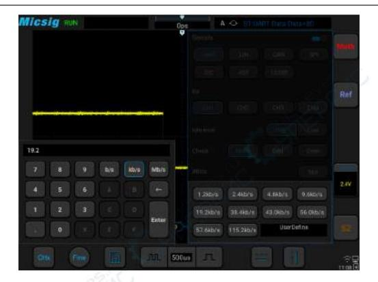
Figure 12-5 Baud Rate Default Setting
