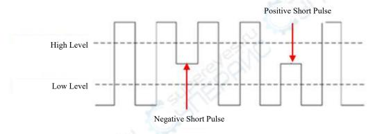
Figure 6-24 Runt Trigger
