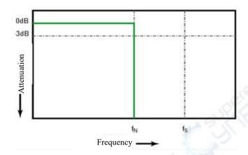
Figure 11-2 Theoretical Brick-Wall Frequency Response
