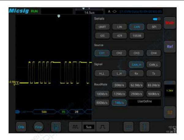
Figure 12-14 CAN Bus Configuration Menu
