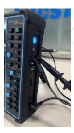
Figure 2-13 Probe Connection
