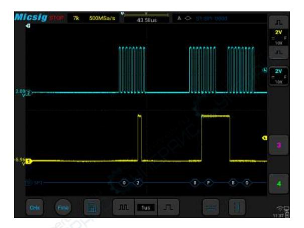
Figure 12-20 SPI Graphic Interface
