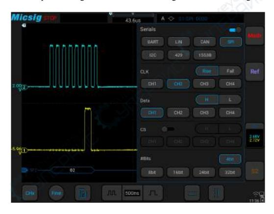
Figure 12-18 SPI Bus Configuration Menu
