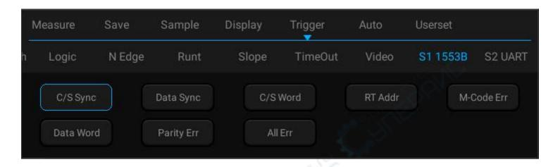
Figure 12-31 1553B Trigger Mode Configuration Menu
