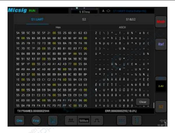
Figure 12-2 Bus Decode Text Mode
