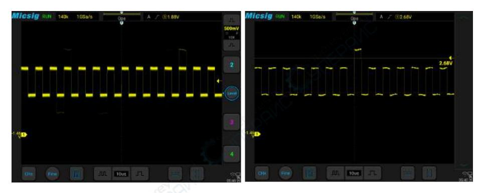
Figure 6-3 Abnormal Signal in Periodic Signals
