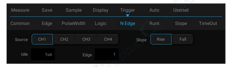
Figure 6-12 Edge Trigger Setting Menu
