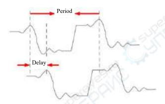
Figure 7-6 Phase Measurement Schematics
