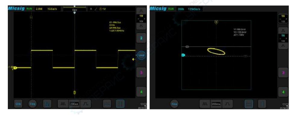
Figure 7-12 Cursor Measurement Pulse Width
