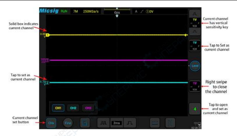
Figure 5-4 Channel Open, Close and Switching
