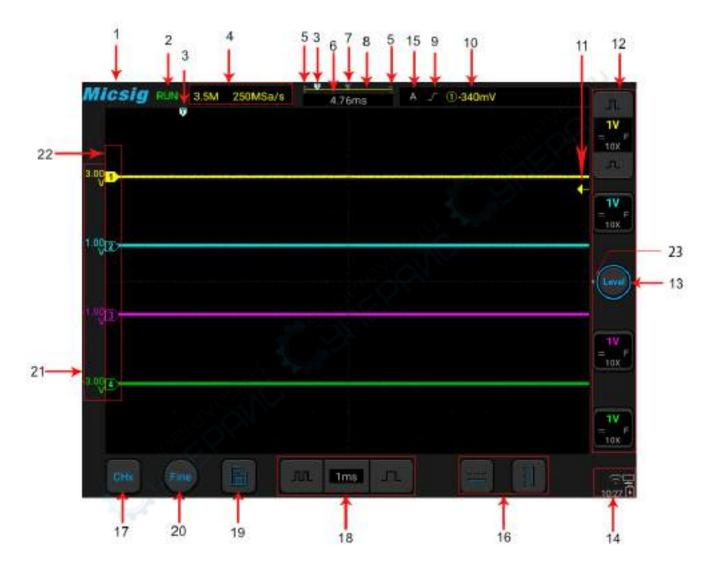
Figure 2-6 Oscilloscope Interface Display
