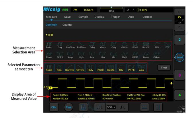
Figure 7-1 Automatic Measurement Menu
