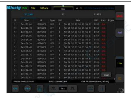
Figure 12-17 CAN Text Interface
