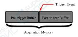
Figure 6-6 Conceptual Demonstration of Acquisition Memory
