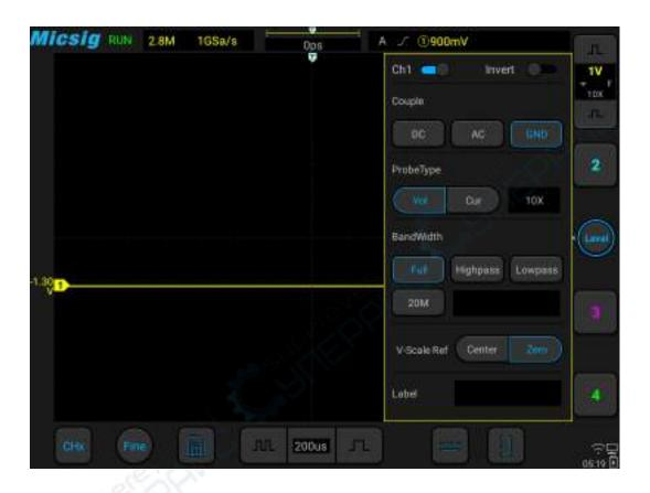
Figure 5-9 GND Coupling
