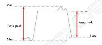
Figure 7-7 Voltage Measurement
