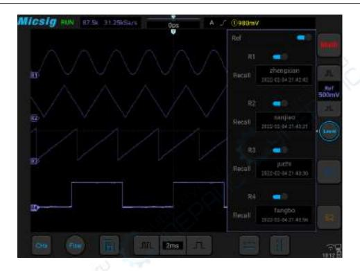
Figure 9-6 Restore Reference Waveform
