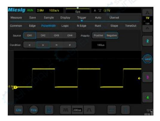
Figure 6-15 Negative Polarity Pulse Level Flip
