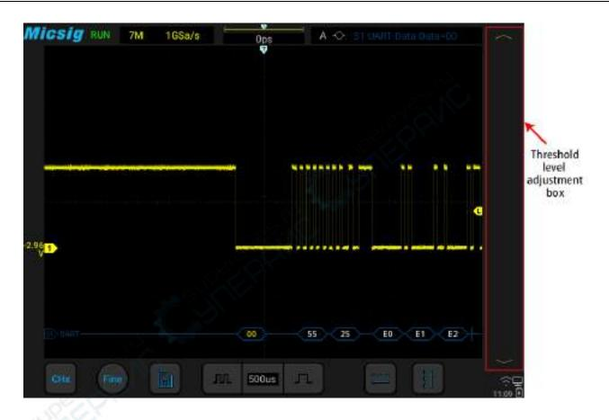
Figure 12-7 UART Decode Level Adjustment
