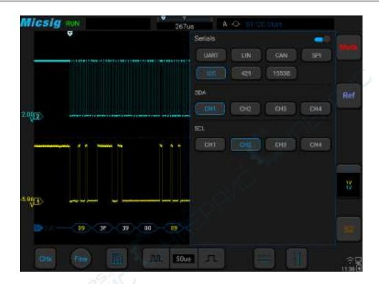
Figure 12-22 I2C Bus Configuration Menu
