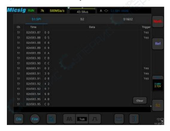
Figure 12-21 SPI Text Interface
