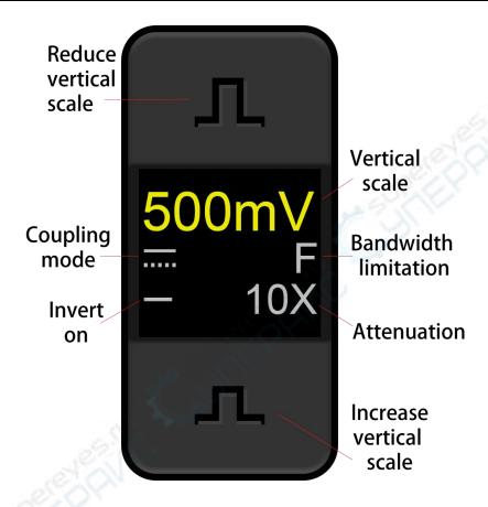
Figure 5-3 Channel Display Interface
