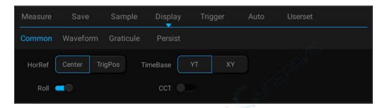
Figure 10-1 Display Settings and Function Buttons
