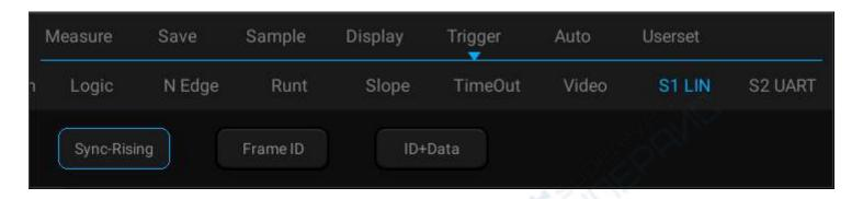
Figure 12-11 LIN Trigger Mode Configuration Menu
