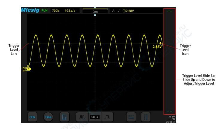
Figure 6-8 Trigger Level
