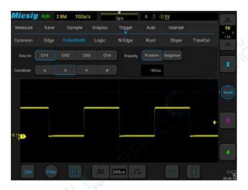
Figure 6-14 Pulse Width Trigger Setting Menu
