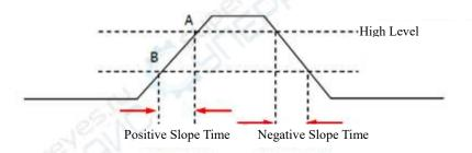
Figure 6-26 Positive/Negative Slope Time
