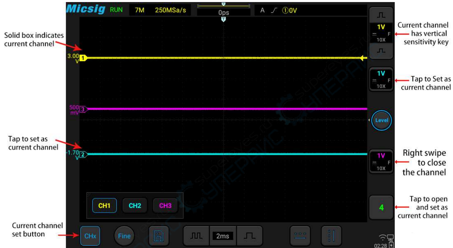
Figure 5-4 Channel Open, Close and Switching
