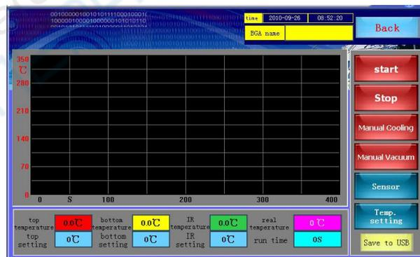
figure13 Operating curve screen
