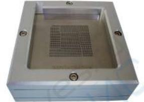
4、 Locking two no spring fixed slide, remove the BGA chip and coated with a thin layer of solder flux, card the chip into the base again, covered with lid(make sure the right direction).
